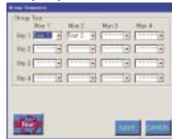
This window is used to edit a group sequence. There are 4 group sequences available, each with up to 4 monitors.
