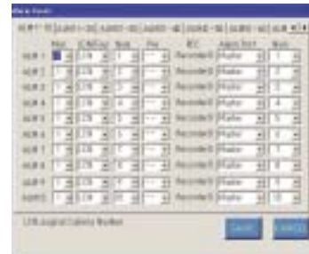
This menu can be used to program which monitor to carry out the spot/tour sequence of which camera, when an alarm signal is input.
